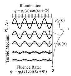
**Fig. 3** Schematic of modulated illumination source (in the *x* direction only) and the resulting modulated internal fluence rate with the same frequency and phase.
