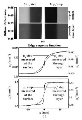
**Fig. 13** Preliminary contrast-resolution study. (a) Gelatin phantoms with a  $3 \times$  step in either absorption (left) or scattering (right) were measured directly (top) and through a 2-mm homogeneous layer (bottom). (b) Edge-response profiles for absorption (top) and scattering (bottom) media reveal loss of both resolution and quantitative contrast through the homogeneous layer (gray lines) compared to that at the surface (black lines).
