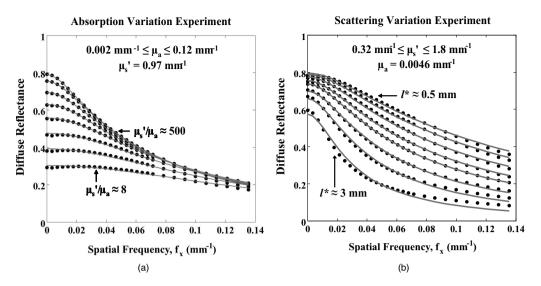
**Fig. 8** Liposyn experiment data (black circles) fit to the SFD diffusion model of Eq. (10) (gray lines). (a) As absorption increases, reflectance at low spatial frequencies decreases dramatically, while high-frequency data shows little sensitivity to absorption contrast. (b) Increasing scattering gives rise to an increase in reflectance, with scattering contrast observed at all frequencies. All results show excellent visual agreement between measurement data and diffusion fits.
