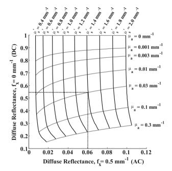
**Fig. 6** Two-frequency (DC versus AC) lookup table for rapid calculation of optical properties, generated from diffusion model forward predictions. Gray contours indicate constant absorption, black contours indicate constant reduced scattering. Dotted lines demonstrate the lookup method, translating DC and AC values into  $\mu_a$  and  $\mu'_s$  parameters.
