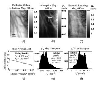
**Fig. 10** (a) Planar diffuse reflectance, (b) optical absorption, and (c) reduced scattering maps. (d) Average multifrequency diffuse reflectance data and least-squares fit to Eq. (10) and pixel histograms of (e) absorption and (f) scattering maps, respectively.
