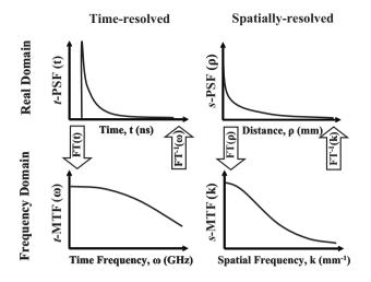
**Fig. 1** Four measurement domains of turbid media characterization: time domain (top left), time frequency domain (bottom left), real spatial domain (top right), and spatial frequency domain (bottom right).
