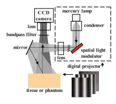
Fig. 2 Modulated imaging instrument platform.
