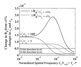
**Fig. 12** Sensitivity of reflectance to 1% change in optical properties for absorption (solid lines) and reduced scattering (dashed lines) optical properties versus normalized spatial frequency. Results indicate that scattering contrast is retained at higher frequencies than absorption contrast. Dotted lines indicate detection thresholds for 12- and 14-bit dynamic range measurements.
