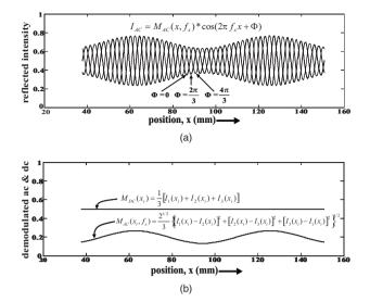
Fig. 5 (a) Schematic of modulated reflectance and (b) demodulated AC and DC amplitudes.
